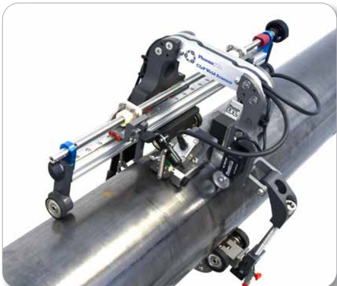
CLiP Weld scanner inspecting a 10" pipe
