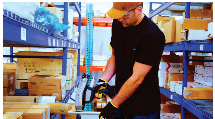
The Niton Apollo in use, verifying incoming materials.
